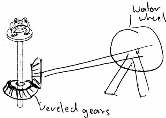
This question, which asked students to add a water wheel to Figure 9, required more abstract thought from students and as a result was worth three marks. For three marks, the water wheel had to be drawn from a side elevation, with a shaft, and the bevel gears drawn at 90 degrees. One or two marks were given to less accurate drawings that essentially met the requirements of the question.
