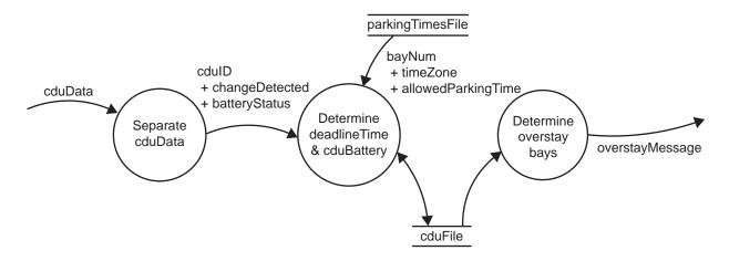
For the process 'Determine deadlineTime & cduBattery' she has developed the following algorithm. It updates deadlineTime and cduBattery in cduFile. The variable currentTime is set by the system and represents the current time of day in 24-hour time.
