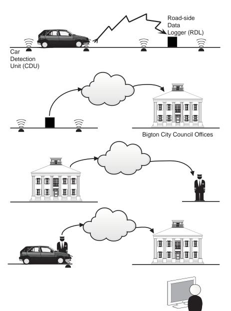
A Car Detection Unit (CDU) in each parking bay detects the arrival (or departure) of a car. When an arrival (or departure) occurs the CDU sends a signal to a nearby Road-side Data Logger (RDL). The signal identifies the CDU and the presence (or absence) of a car.
