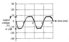
The output varied about zero, was inverted, had the same frequency as the original and was clipped at +8 and -12 V.
