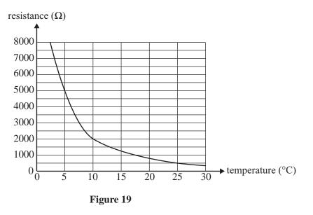
What is the resistance of the thermistor when the temperature is 5 °C?
