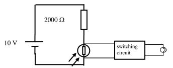
Common errors included placing the switching circuit in series with the battery, resistor and LDR. This was unusual given the relatively standard circuit design required in this type of circuit. Another common error was connecting the switching circuit in parallel with the resistor.
