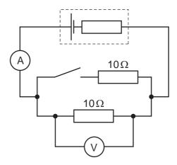
The cell has an e.m.f. of 1.5 V. The voltmeter reads 1.2 V when the switch is open.
