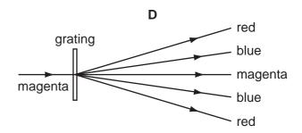
**32** Light produced by a calcium discharge lamp strikes a diffraction grating, with 800 slits per mm, at right angles to the surface.
