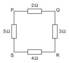
Between which points will the ohmmeter reading be the smallest?
