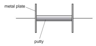
With the putty arranged like this, it has a resistance of  $8\Omega$ .
