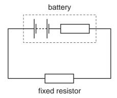
The battery is replaced by one of the same e.m.f. but with a larger internal resistance.
