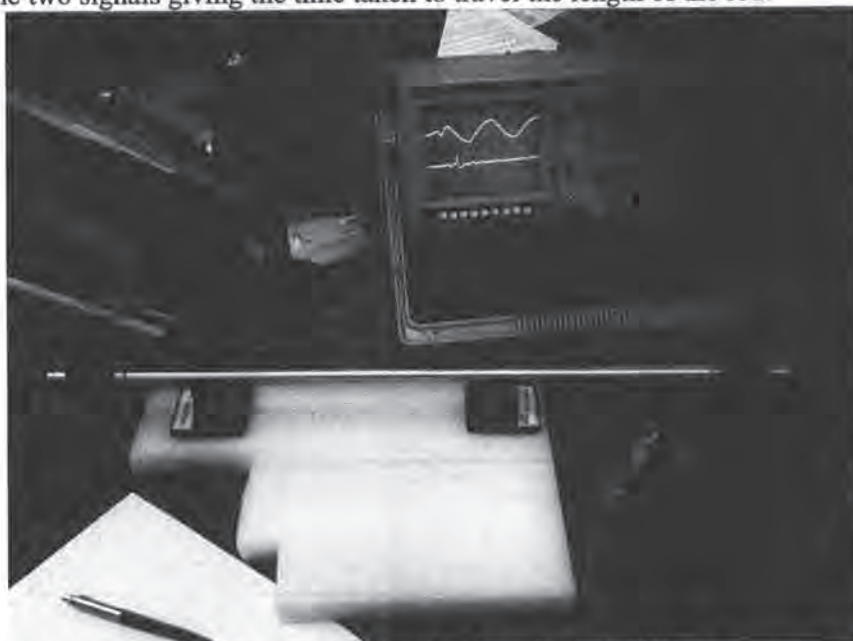
Set up to measure speed of sound in aluminium
