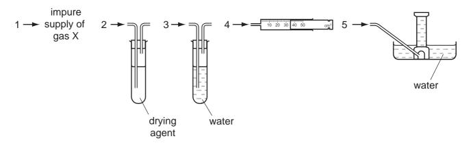
In which order should pieces of apparatus be joined together to collect a pure, dry sample of X?
