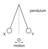
Which sequence should be timed to measure the period of the pendulum?
