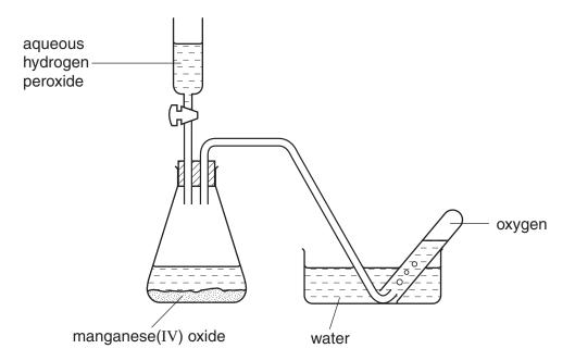
The first few test-tubes of collected gas should be rejected because the oxygen would be contaminated by
