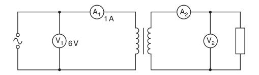
Which pair of readings are possible on meters  ${\rm V_2}$  and  ${\rm A_2}$ ?
