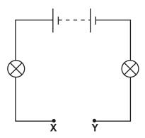
Which component can be connected between **X** and **Y** so that the brightness of the lamps may be varied?
