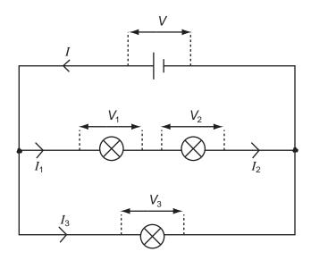
Which pair of equations is correct for this circuit?
