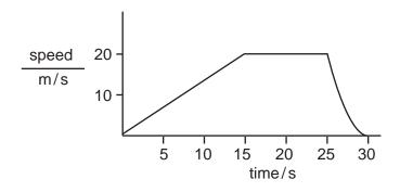
How far does the car travel before the brakes are applied?
