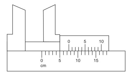
What reading is shown on the vernier calipers?
