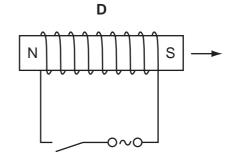
magnet withdrawn before switching off
