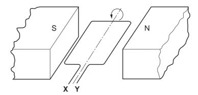
When the coil is part of an a.c. generator, what must be connected directly to **X** and **Y**?
