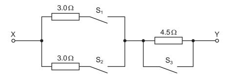
Which switch positions give a resistance of  $6.0 \Omega$  between X and Y?
