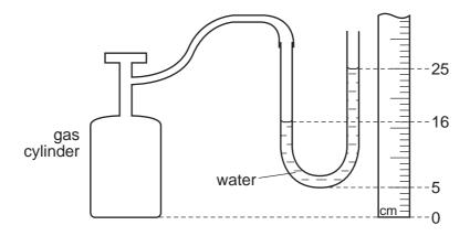
What is the pressure difference, in cm of water, shown by the manometer?
