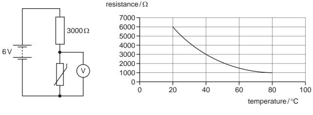
What is the temperature of the thermistor when the voltmeter reads 2V?
