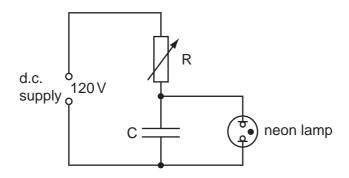
The neon lamp lights when the p.d. across the capacitor C reaches 110V. C then discharges through the neon lamp. When C has discharged, the lamp goes out and the p.d. across C slowly increases once more.
