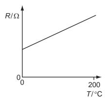
The resistance of the wire at  $0 \degree C$  is  $1.00 \Omega$  and at  $100 \degree C$  is  $1.40 \Omega$ .
