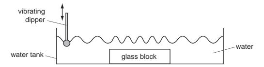
What happens to the frequency and to the speed of the wave as it reaches the glass block?
