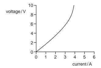
The voltage across the lamp increases. What happens to the temperature of the lamp and the resistance of the lamp?
