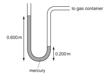
The density of mercury is  $13600 \text{ kg/m}^3$ . The gravitational field strength *g* is 10 N/kg. What is the pressure difference between the gas in the container and the atmosphere? **A** 27200 Pa **B** 40800 Pa **C** 54400 Pa **D** 81600 Pa
