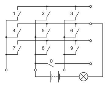
Which single switch can be pressed to make the lamp light?
