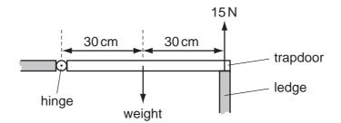
When the trapdoor is closed, the ledge exerts an upward force of 15 N on the trapdoor. The gravitational field strength is 10 N/kg.
