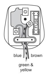
What is the effect of using the plug wired in this way?
