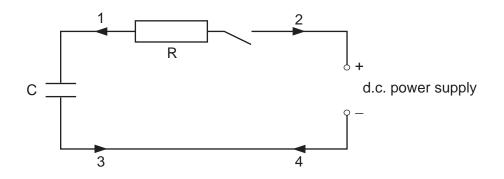
Which arrows show the direction of the conventional current when the capacitor is charging?
