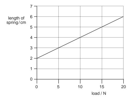
A load causes the spring of the balance to extend by 3 cm.
