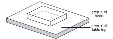
The area of the block in contact with the table is X and the area of the table top is Y.
