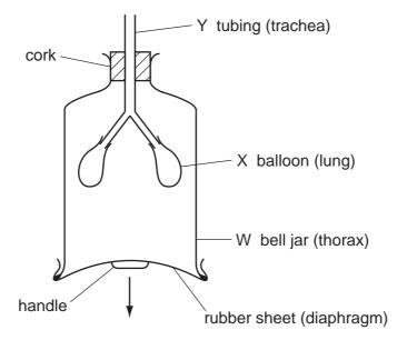
The handle is pulled down moving the rubber sheet in the direction of the arrow.
