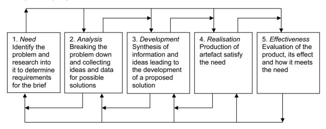
The arrows show that it is not always a linear series, that there is frequent looping back, particularly an ongoing reappraisal of the nature of the need. The arrows at the top showing forward links indicate for example that when considering the nature of the need (box 1) the resources available for realisation (box 4) and the constraints must be kept in mind. Similarly, the likely effects (box 5) need to be anticipated at every stage.
