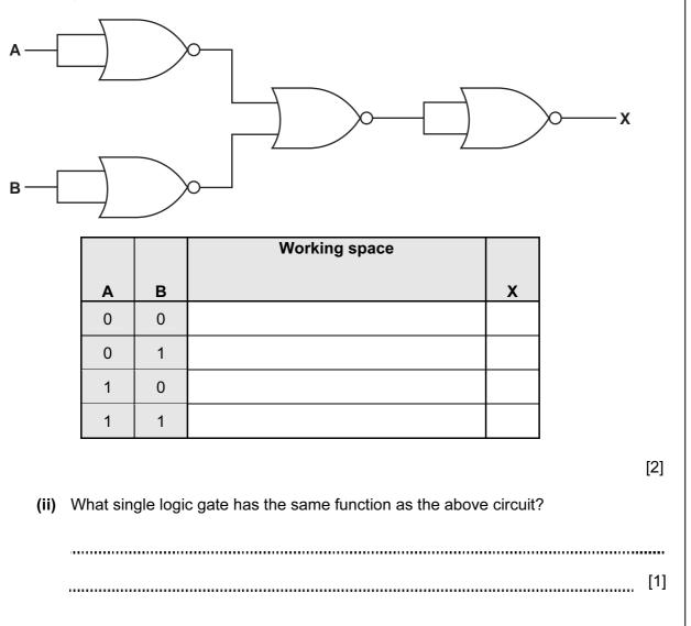
(b) Complete the truth table for the following logic circuit.
