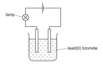
Why does the lamp light up only when the lead(II) bromide is melted?
