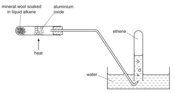
The ethene is then tested with aqueous bromine.
