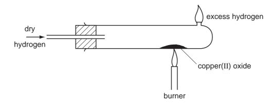
Why is the hydrogen allowed to flow through the tube during cooling?
