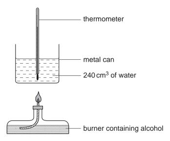
Some butan-1-ol was put into the burner, which was weighed. The temperature of the water was noted. The burner was lit and allowed to burn for several minutes. The flame was extinguished and the final temperature of the water was noted. The burner was reweighed.
