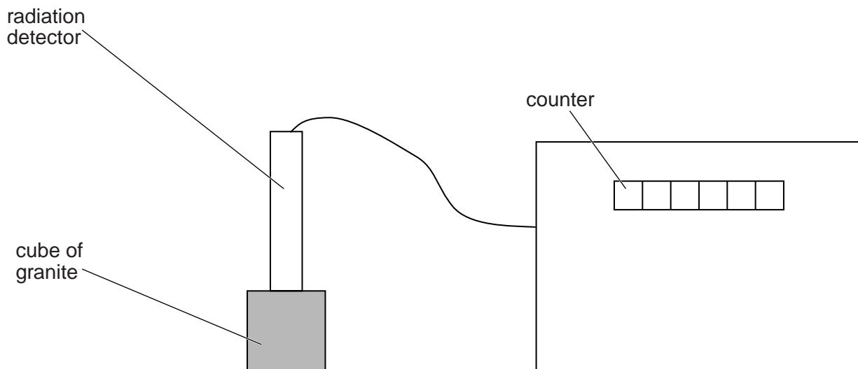
The counter records how many radioactive counts are received from the detector.
