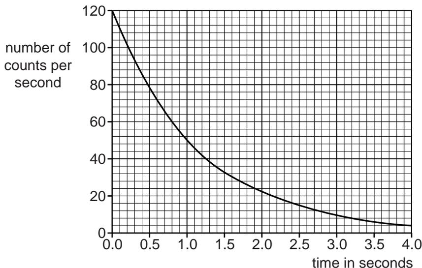
(i) Before the graph was plotted, the background radiation count was removed from the readings so that the graph shows only the radiation from the helium-6.
