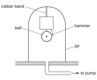
The pump is switched on and the air is removed from the jar. The hammer still hits the bell but the sound becomes quieter until it cannot be heard.
