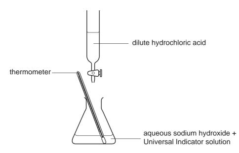
Dilute hydrochloric acid is run from a burette into the flask until a neutral solution is formed.
