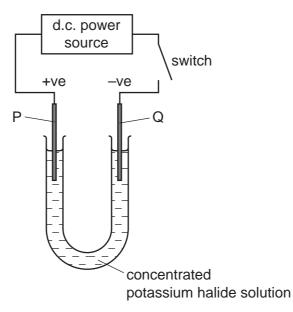
When the switch is closed, the solution near electrode P turns brown because a halogen is formed.
