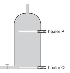
When only heater Q is switched on, it takes a long time to heat the tank of water to the required temperature of 60 °C.
