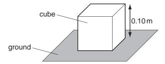
The cube weighs 200 N and its sides are 0.10 m long.
