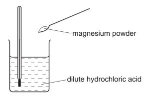
Thermometer reading before adding magnesium powder = 20.6 °C
