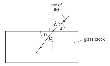
Which of the labelled angles is the angle of refraction?
