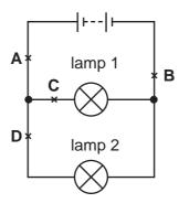
At which labelled point should a switch be placed so that lamp 1 remains on all the time and lamp 2 can be switched on and off?
