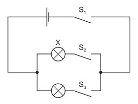
Which switches will have to be closed so that only bulb X will light?
