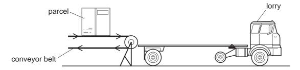
The parcel travels towards the lorry at a constant speed. Only two horizontal forces act on the parcel: air resistance, and friction with the conveyor belt.
