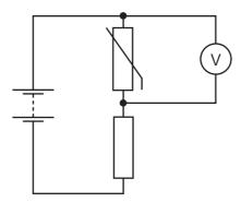
The temperature of the thermistor increases.
