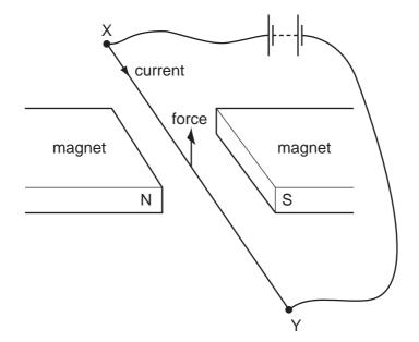
If the north and south poles of the magnet exchange positions, in which direction will the force on the wire act?
