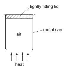
When the can is heated strongly behind a safety screen, the lid is blown off by the increased pressure inside the can.
