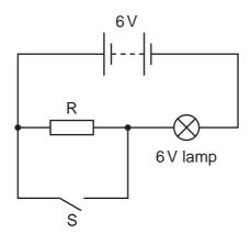
What happens to the brightness of the lamp when switch S is closed?
