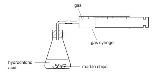
The experiment is repeated using  $2\,\mathrm{g}$  of marble chips and an excess of  $2\,\mathrm{mol}\,/\,\mathrm{dm}^3$  hydrochloric acid.
