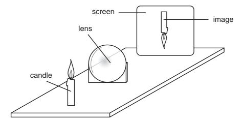
The screen and the lens are moved back and forth and various focused images are produced on the screen.
