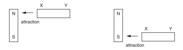
How does end Y behave when it is placed, in turn, near to the two poles of the magnet?
