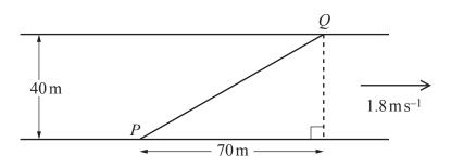
The diagram shows a river with parallel banks. The river is 40 m wide and is flowing with a speed of  $1.8 \text{ ms}^{-1}$ . A canoe travels in a straight line from a point *P* on one bank to a point *Q* on the opposite bank 70 m downstream from *P*. Given that the canoe takes 12 s to travel from *P* to *Q*, calculate the speed of the canoe in still water and the angle to the bank that the canoe was steered. [8]
