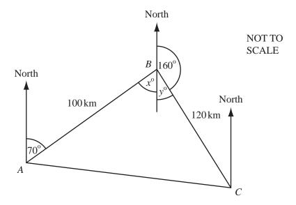
A ship sails 100 kilometres from A on a bearing of  $070^{\circ}$  to B. It then sails 120 kilometres on a bearing of  $160^{\circ}$  to C.
