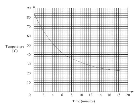
The graph shows the temperature of a cup of tea cooling down in a room.
