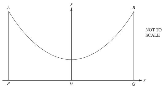
The diagram shows two vertical poles (AP and BQ) that support the ends (A and B) of a hanging chain. The chain is symmetrical about the *y*-axis.
