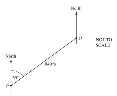
The diagram shows a straight road PQ. PQ = 840m and the bearing of Q from P is  $065^{\circ}$ .
