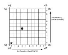
To give the six figure grid reference, first of all identify the grid square, in this case 4665. The third figure is obtained by dividing the space between grid lines 46 and 47 into ten equal parts. Similarly the sixth figure is obtained by a similar division of the gap between northings 65 and 66. This would result in a grid reference of 463654 for the dot and 460650 for the star. It should be noted that the first tenth is 0 and the last tenth is 9 in the divided grid square.
