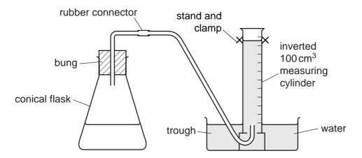
Using a measuring cylinder,  $50 \text{ cm}^3$  of dilute acid **X** was poured into the conical flask. 0.5g of magnesium ribbon was added to the conical flask and the bung added.
