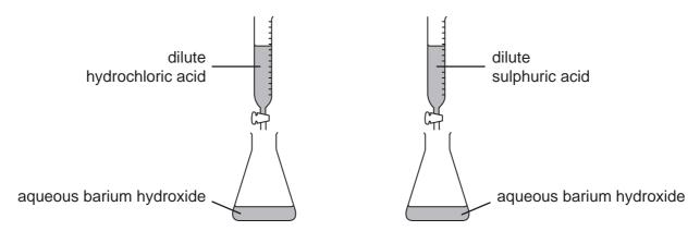
In each experiment, the acid is run into the conical flask until the resulting liquid has pH7.
