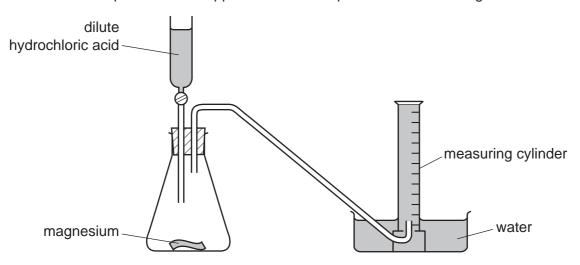
Using a tap funnel, 20 cm<sup>3</sup> of hydrochloric acid was added to 4 cm of magnesium ribbon. The volume of hydrogen produced was measured every minute for six minutes.
