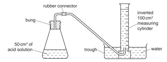
Using a measuring cylinder, 50 cm<sup>3</sup> of acid **X** was poured into the conical flask. 0.5 g of magnesium ribbon was added to the conical flask and the bung replaced.
